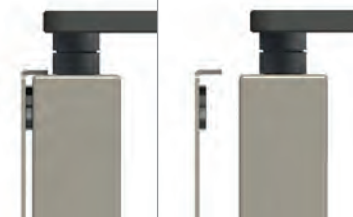
mounting by magnets and small hooks
