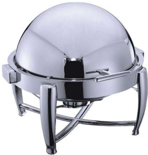
Chafing Dish With Plain Lid,36cm Pan 6L A-1031S SS304 540x500xH478mm All of the chafing dishes are made of 304 Stainless Steel. There is a water return system, condensation flows back to water pan instead of food.RollTop for Banquet. stackable design.
